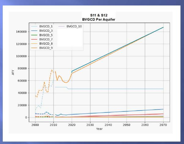
Run S11 and S12 Simsboro (Layer 9) Slight Pumping Modification Pumping from All of the Aquifers in all other areas of the model the same for S-11 and S-12
