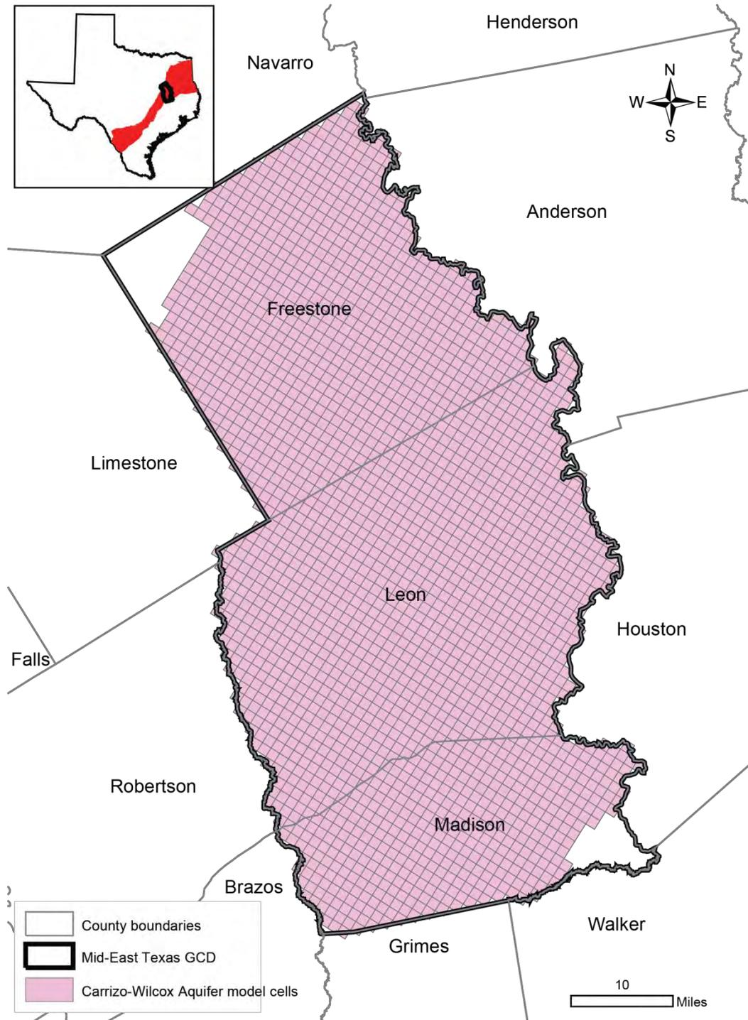
**FIGURE 4: AREA OF THE GROUNDWATER AVAILABILITY MODEL FOR THE CARRIZO-WILCOX AQUIFER FROM WHICH THE INFORMATION IN TABLE 4 WAS EXTRACTED. ONLY THE CELLS REPRESENTING THE CARRIZO-WILCOX AQUIFER WITHIN THE DISTRICT BOUNDARIES ARE SHOWN.**
