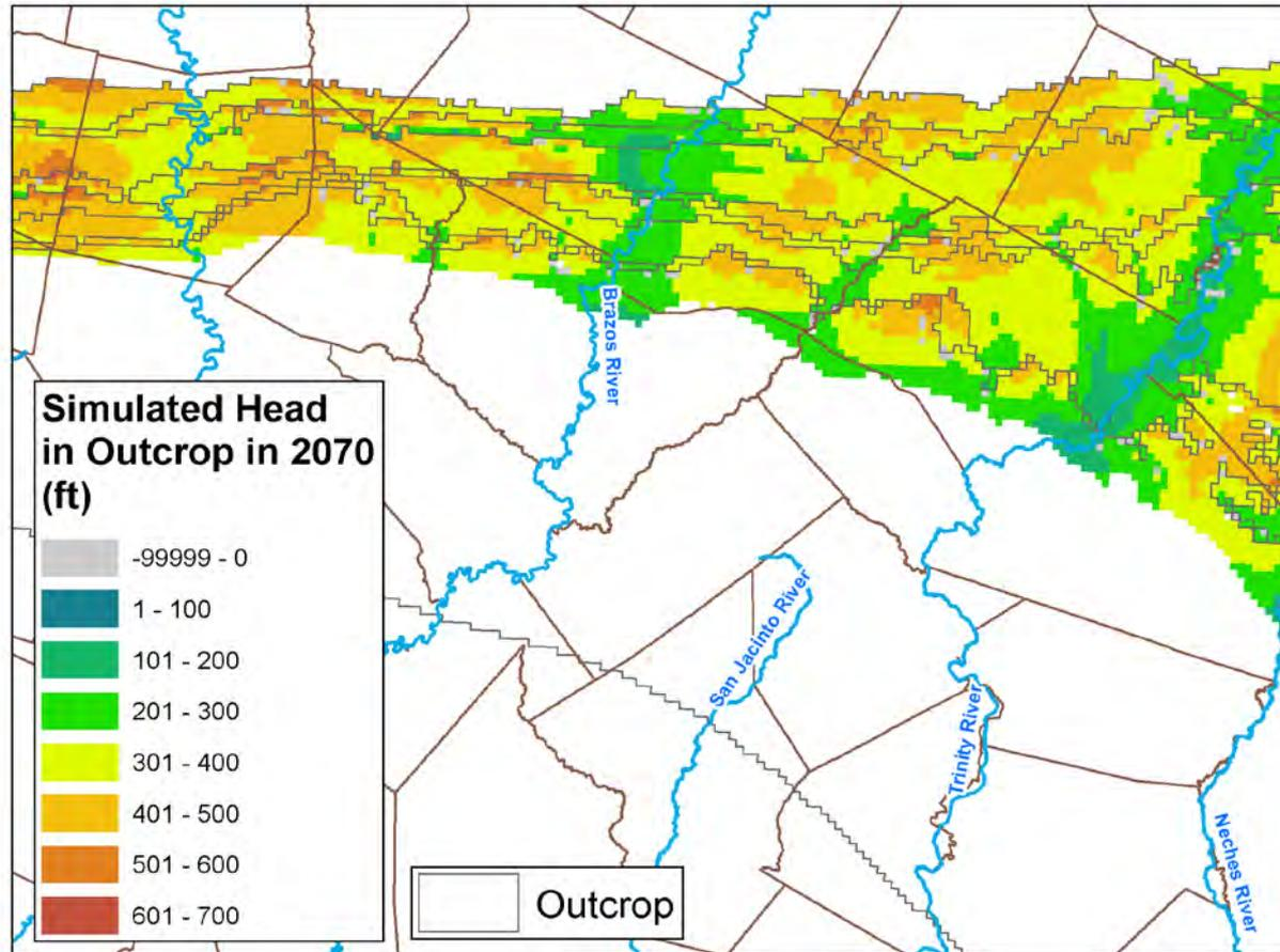
**Note:** In the aquifer outcrop, there is strong correlation between the model layering and outcrop location and the water table elevation
