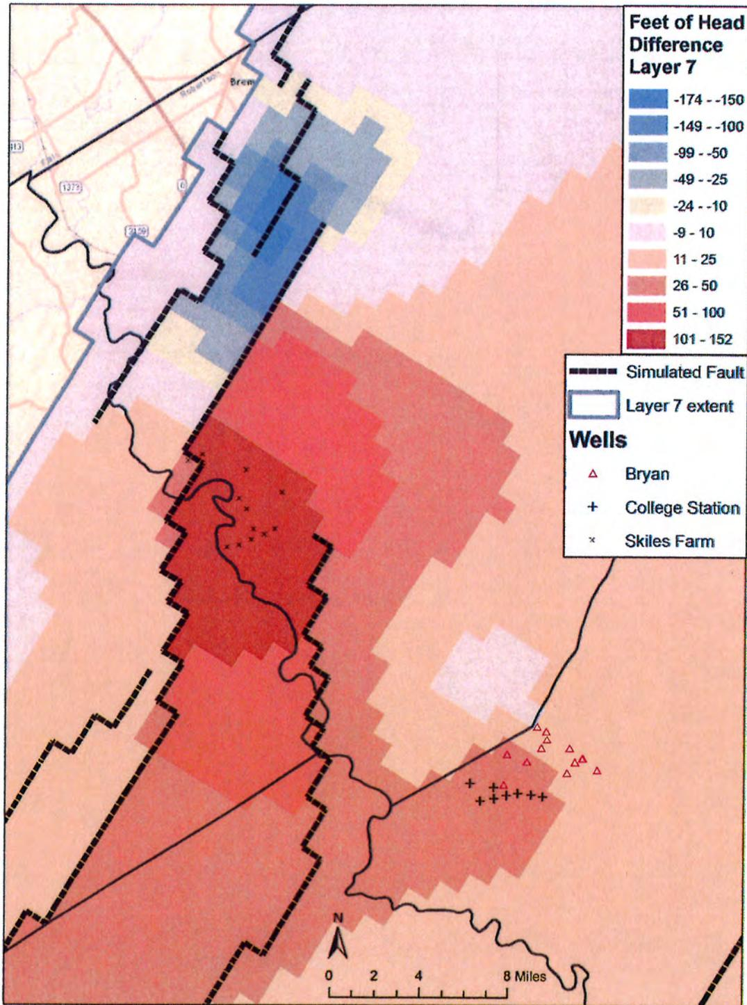
**Figure 5.** Map showing the difference between simulated Simsboro Aquifer heads in PS6 and PS6\_mod in 2070. The values represent the difference between PS6 and PS6\_mod, so that negative values indicate higher heads (less drawdown) in PS6\_mod, while positive values indicate more drawdown in PS6\_mod.
