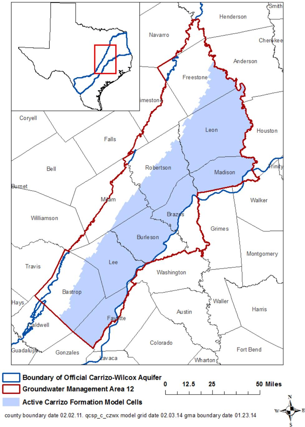
**FIGURE 12. EXTENT OF THE GROUNDWATER AVAILABILITY MODEL FOR THE CENTRAL PART OF THE CARRIZO-WILCOX, QUEEN CITY, AND SPARTA AQUIFERS USED TO ESTIMATE TOTAL RECOVERABLE STORAGE FOR THE CARRIZO FORMATION (TABLES 21 AND 22) WITHIN GROUNDWATER MANAGEMENT AREA 12.**
