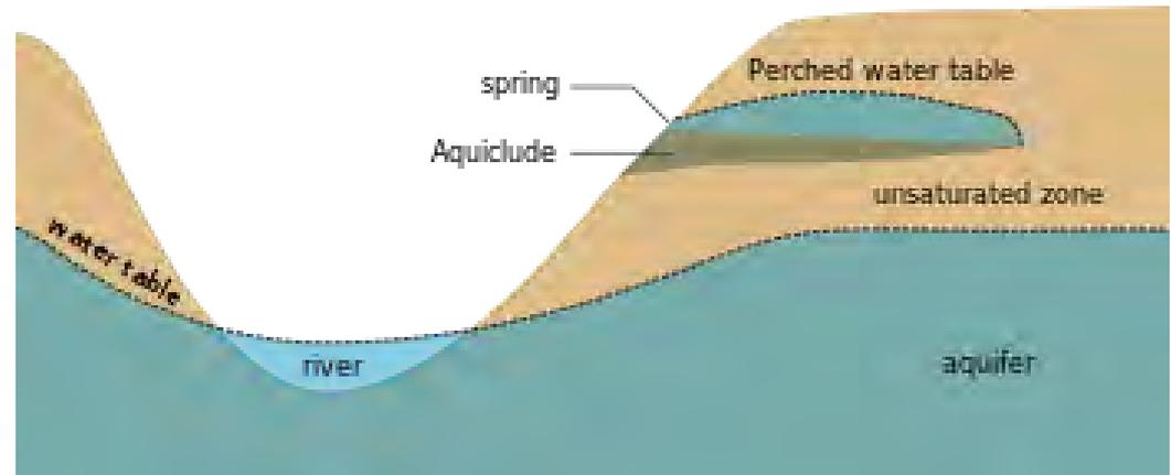
**Schematic of a spring connected to a perched water table ( 2015,[https://en.wikipedia.org/wiki/Water\\_table](https://en.wikipedia.org/wiki/Water_table))**
