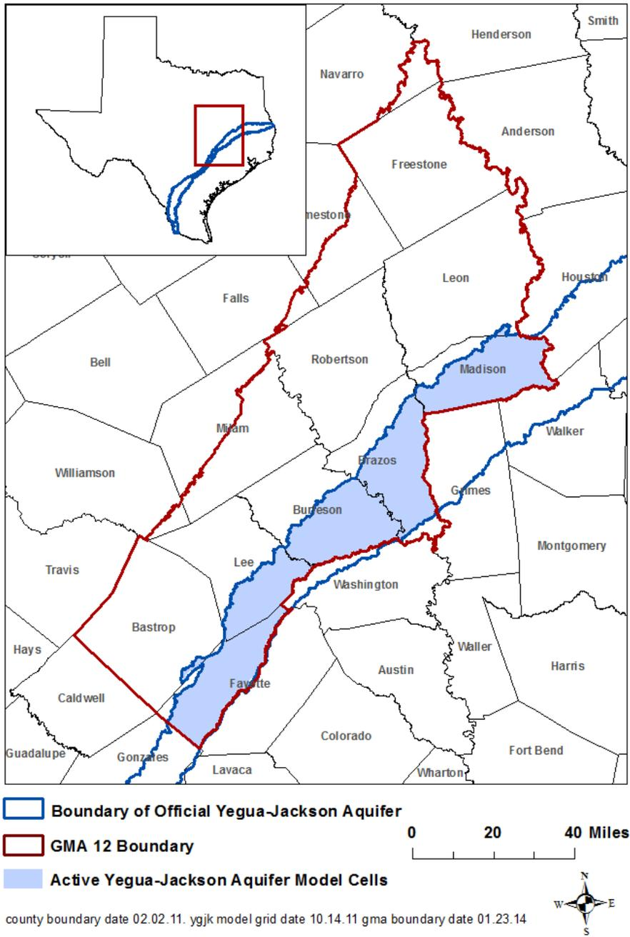
**FIGURE 6. EXTENT OF THE GROUNDWATER AVAILABILITY MODEL FOR THE YEGUA-JACKSON AQUIFER USED TO ESTIMATE TOTAL RECOVERABLE STORAGE (TABLES 9 AND 10) FOR THE YEGUA-JACKSON AQUIFER WITHIN GROUNDWATER MANAGEMENT AREA 12.**
