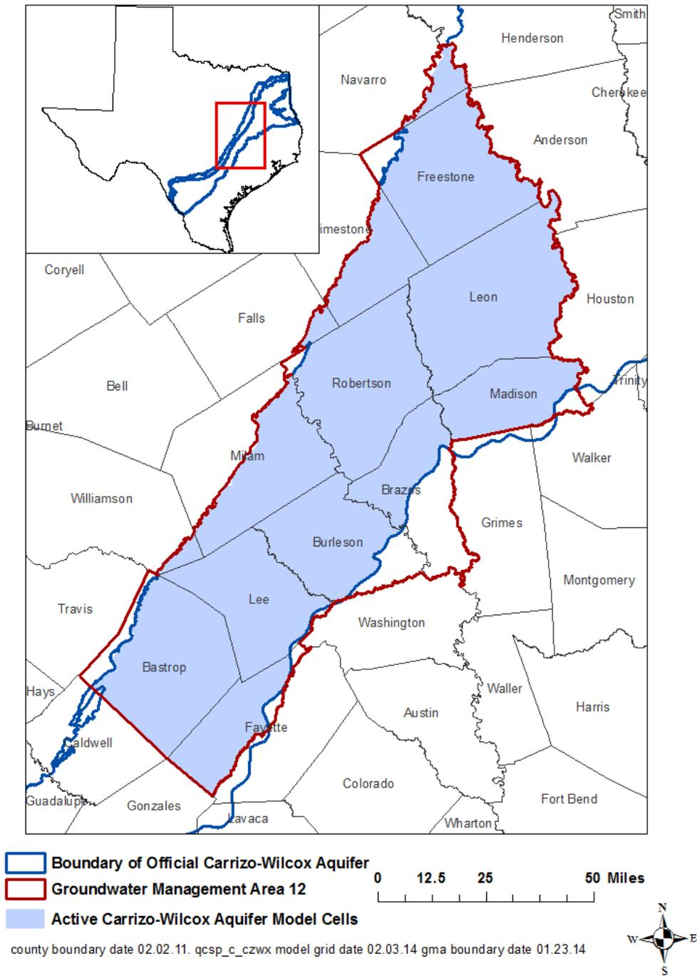
**FIGURE 3. EXTENT OF THE GROUNDWATER AVAILABILITY MODEL FOR THE CENTRAL PART OF THE CARRIZO-WILCOX, QUEEN CITY, AND SPARTA AQUIFERS USED TO ESTIMATE TOTAL RECOVERABLE STORAGE FOR THE CARRIZO-WILCOX AQUIFER (TABLES 3 AND 4) WITHIN GROUNDWATER MANAGEMENT AREA 12.**
