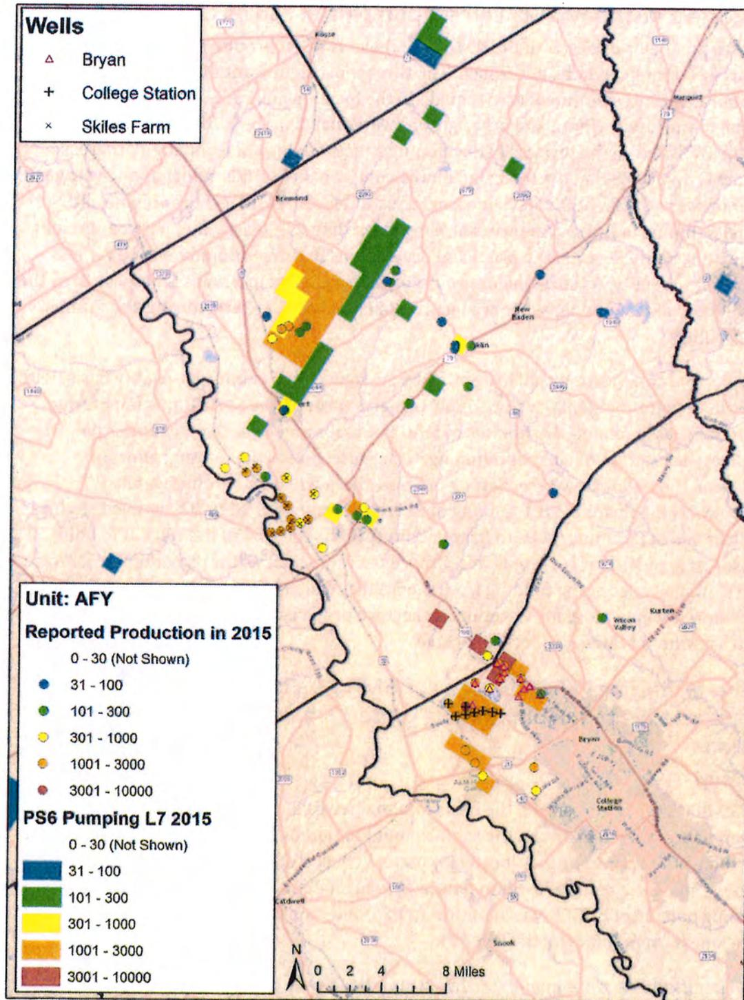
**Figure 2.** Map comparing location and annual volume of reported and simulated groundwater production from the Simsboro Aquifer in BVGCD in 2015. Reported production compiled from BVGCD reported water production data. PS6 pumping extracted from PS6 pumping input file.
