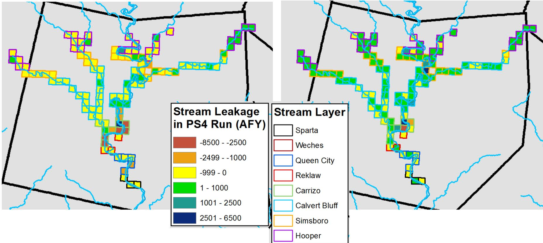
**Note: Negative flows (red, orange, yellow) means the aquifer is providing groundwater to the stream – so stream is gaining. Positive flows (greens and blues) means the aquifer is receiving water from the stream – so stream is losing.**
