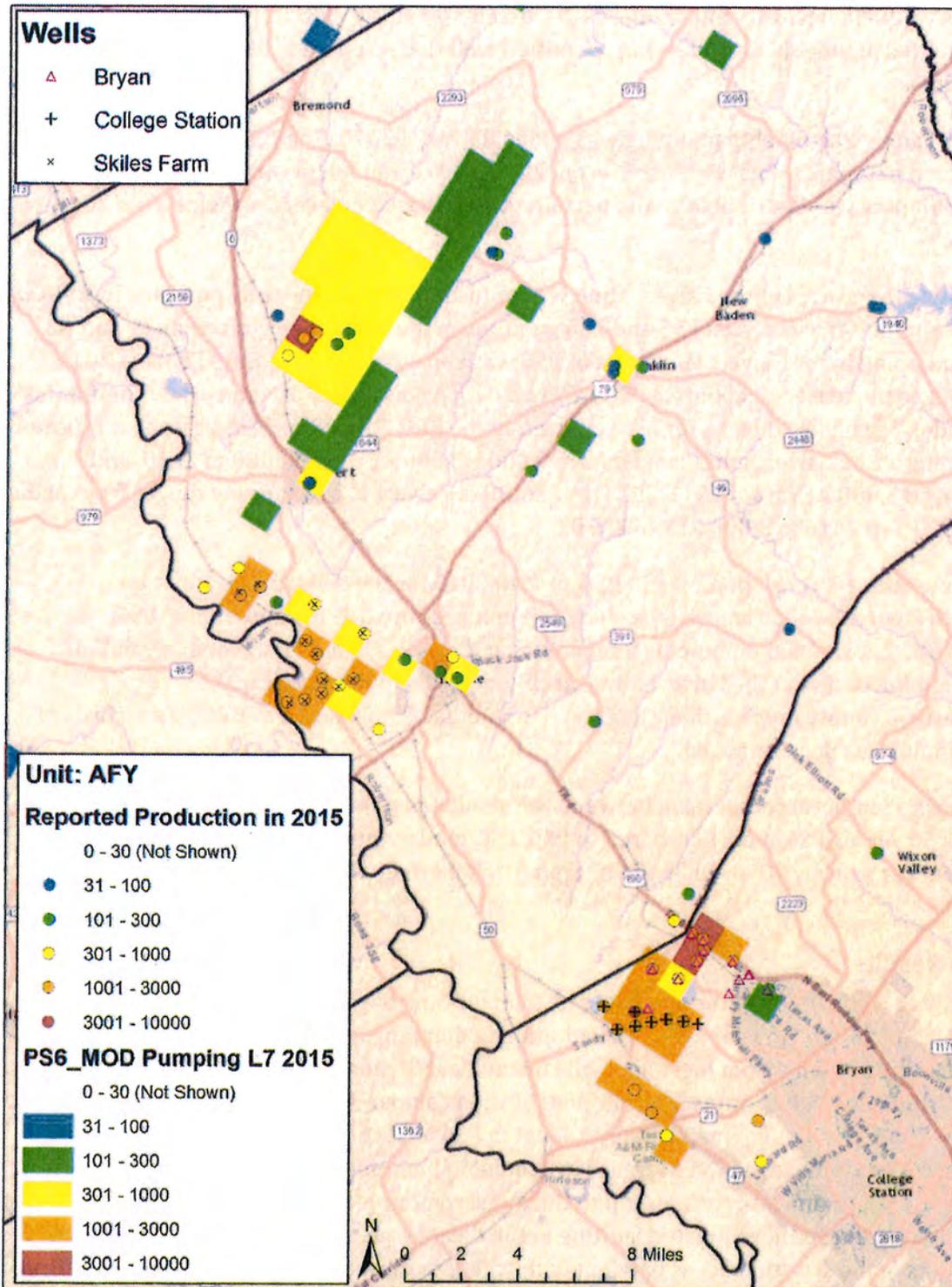
**Figure 3.** Map comparing location and annual volume of reported and modified simulated groundwater production from the Simsboro Aquifer in BVGCD in 2015. Reported production compiled from BVGCD reported water production data. PS6\_mod pumping extracted from PS6\_mod pumping input file.
