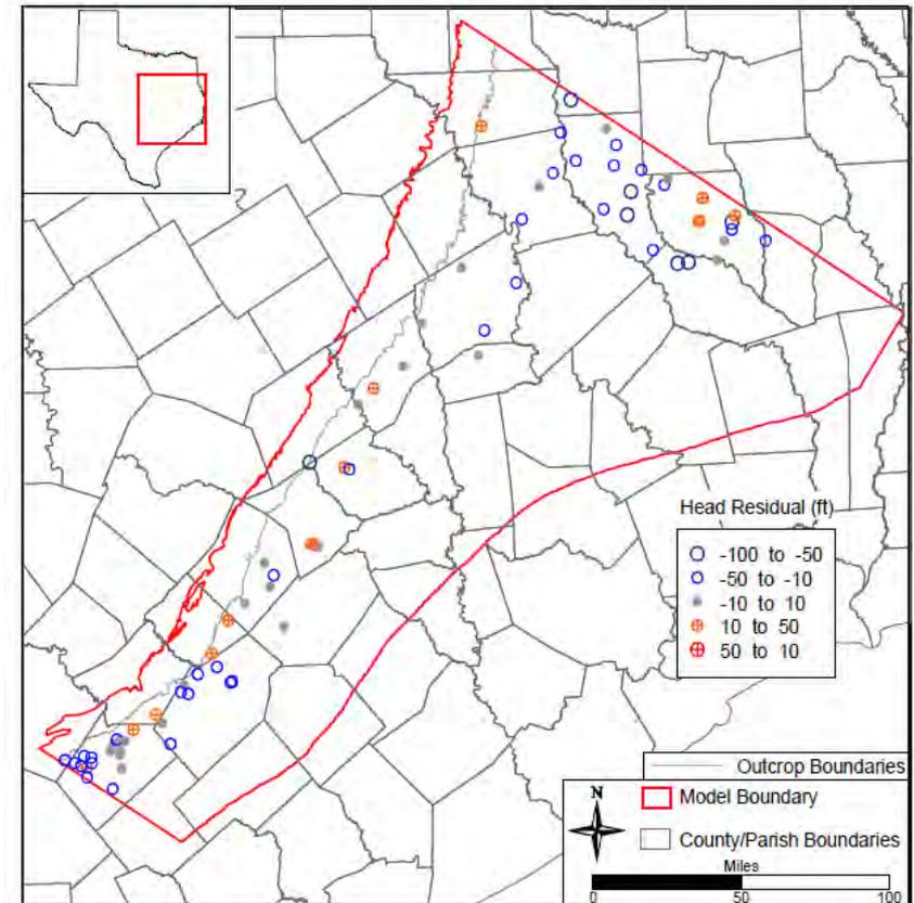
Head Residual = Modeled Head – Measured Head
