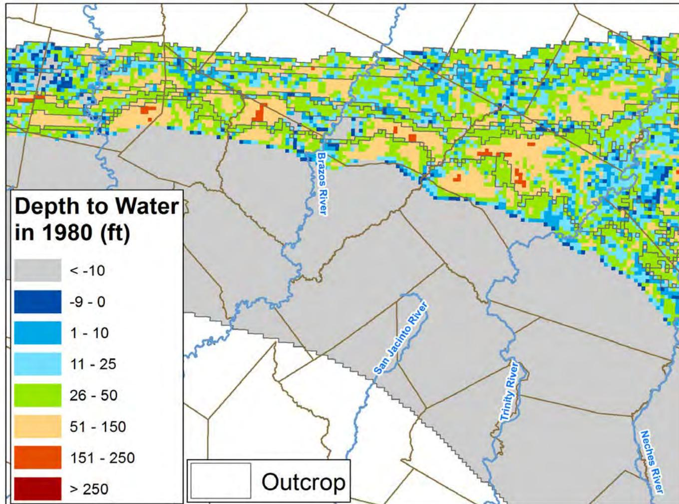
**Note: In down-dip reaches of some of the aquifer outcrops, the depth to the water table exceeds 150 feet in 1980**
