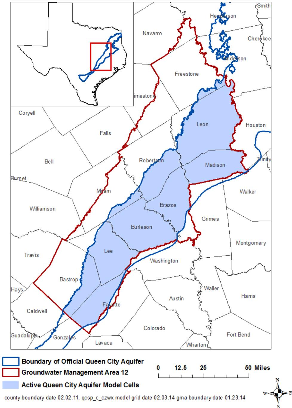
**FIGURE 4. EXTENT OF THE GROUNDWATER AVAILABILITY MODEL FOR THE CENTRAL PART OF THE CARRIZO-WILCOX, QUEEN CITY, AND SPARTA AQUIFERS USED TO ESTIMATE TOTAL RECOVERABLE STORAGE FOR THE QUEEN CITY AQUIFER (TABLES 5 AND 6) WITHIN GROUNDWATER MANAGEMENT AREA 12.**
