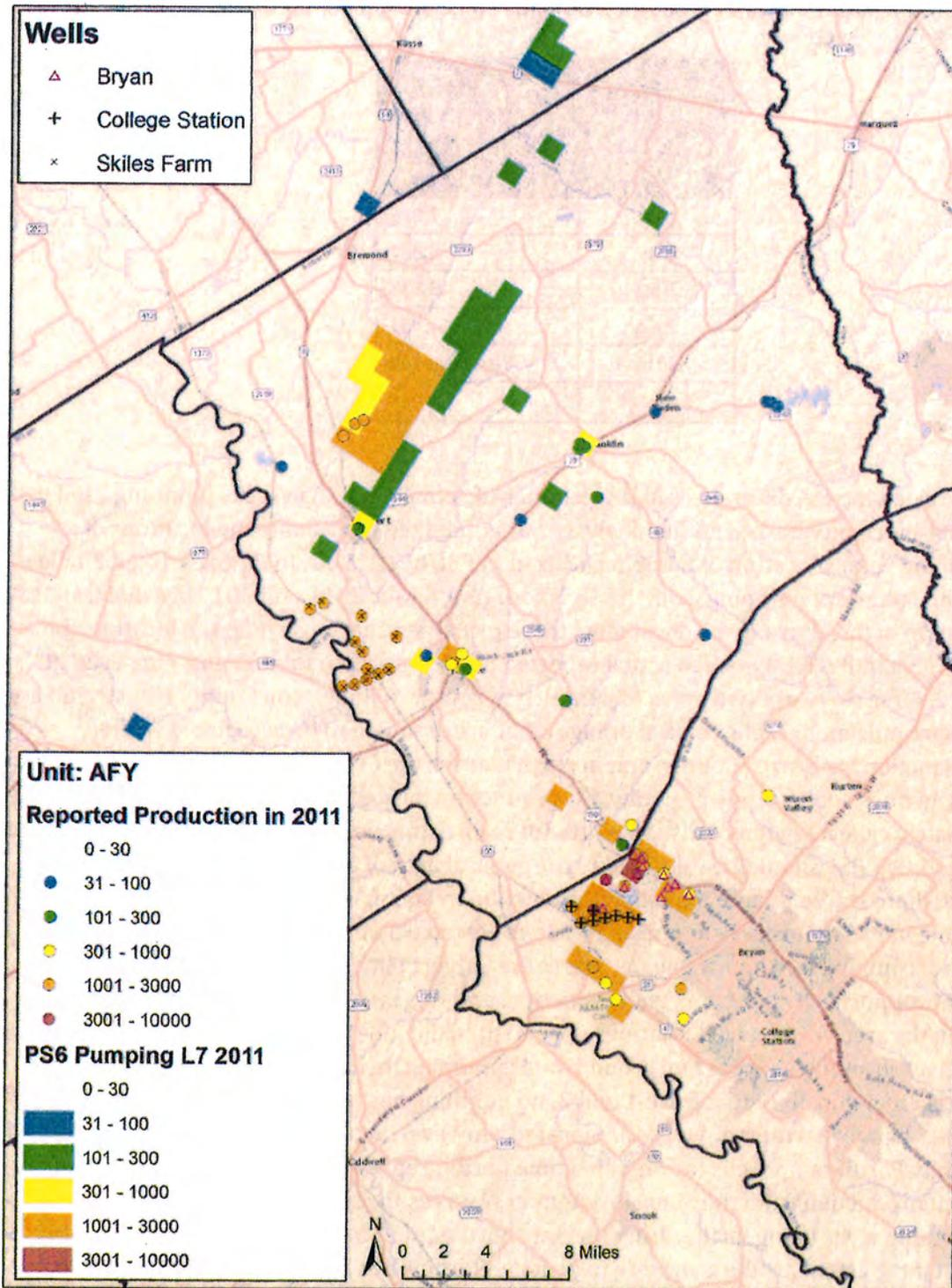
**Figure 1.** Map comparing location and annual volume of reported and simulated groundwater production from the Simsboro Aquifer in BVGCD in 2011. Reported production compiled from BVGCD reported water production data. PS6 pumping extracted from PS6 pumping input file.
