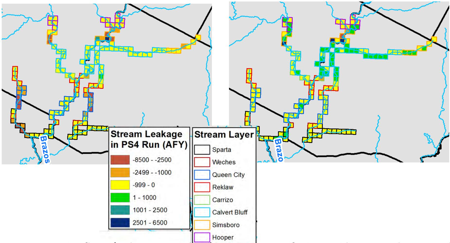
**Note: Negative flows (red, orange, yellow) means the aquifer is providing groundwater to the stream – so stream is gaining. Positive flows (greens and blues) means the aquifer is receiving water from the stream – so stream is losing.**
