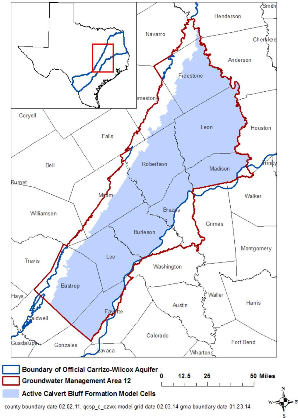
**FIGURE 11. EXTENT OF THE GROUNDWATER AVAILABILITY MODEL FOR THE CENTRAL PART OF THE CARRIZO-WILCOX, QUEEN CITY, AND SPARTA AQUIFERS USED TO ESTIMATE TOTAL RECOVERABLE STORAGE FOR THE CALVERT BLUFF FORMATION (TABLES 19 AND 20) WITHIN GROUNDWATER MANAGEMENT AREA 12.**
